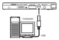
When connected to a computer, a pop-up window appears on this unit's display to let you choose whether you want to operate the unit using USB bus power or to connect the unit with the computer by USB.
